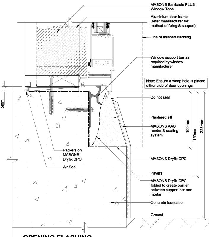
**OPENING FLASHING -CONCRETE DOOR SILL** With Rebate
