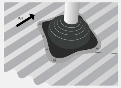
Fit roof boot flashing on diagonal and seal and fix to roofing profile
