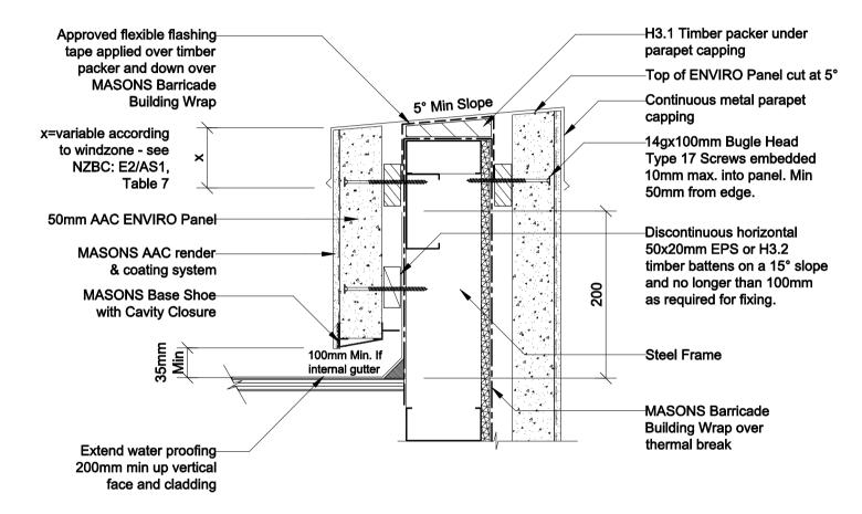
PARAPET CONSTRUCTION -Metal Capping
