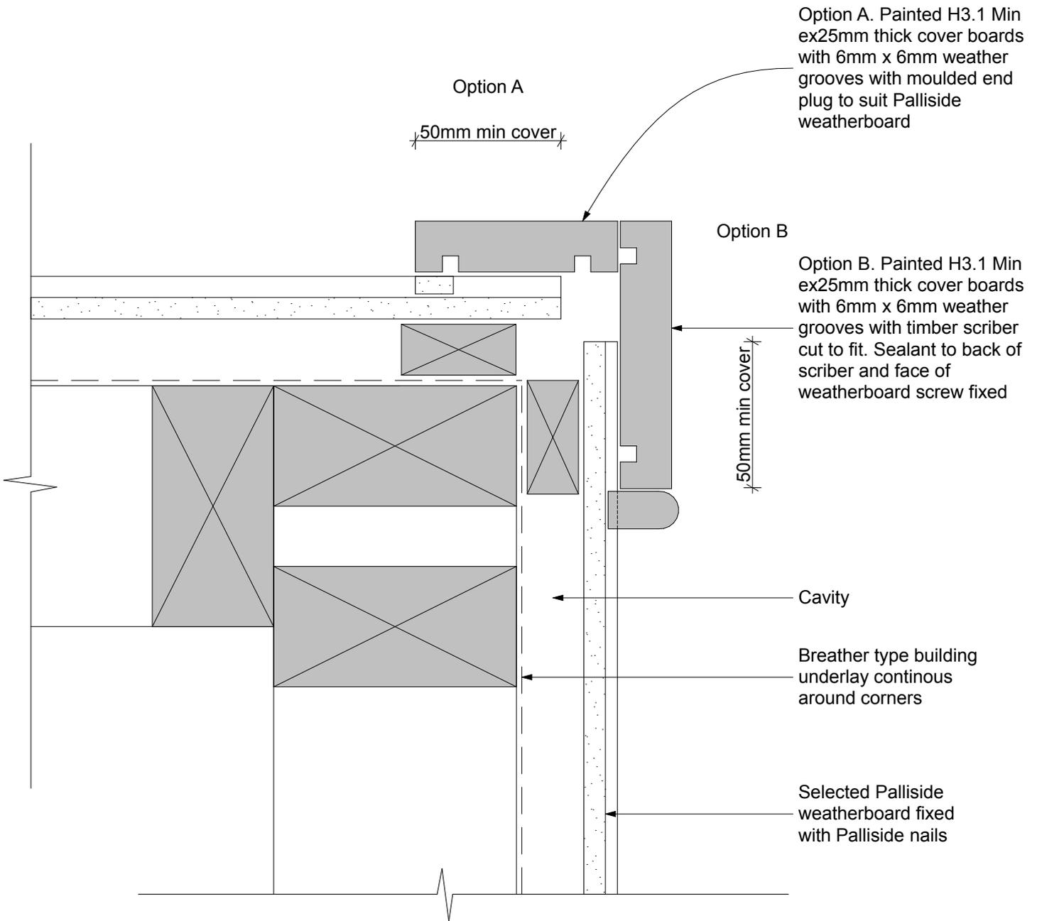
Cover boards shall be sized to provide 50mm min cover over cladding
