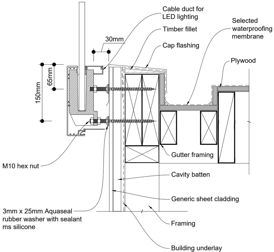
M10 Lag screws must have 90mm penetration into double joist
