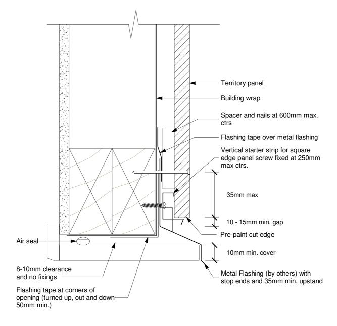
Note: Vertical sealant filled joints must be provided at sides of opening
