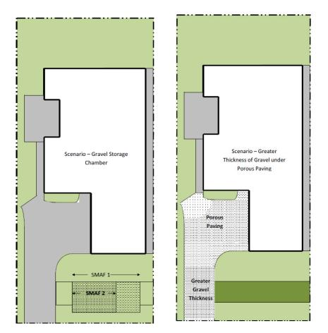
Figure 2-2 Single House Stormwater Management Scenarios (D&B Kettle Consulting Ltd 2013a)
