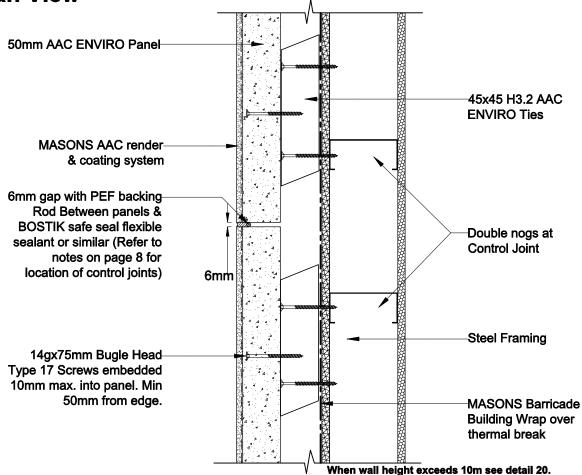
**CONTROL JOINTS - HORIZONTAL Detail 19** Scale 1:5 Section View Note: Refer to page 8 Section Control Joints Re: For the placement of control joints.
