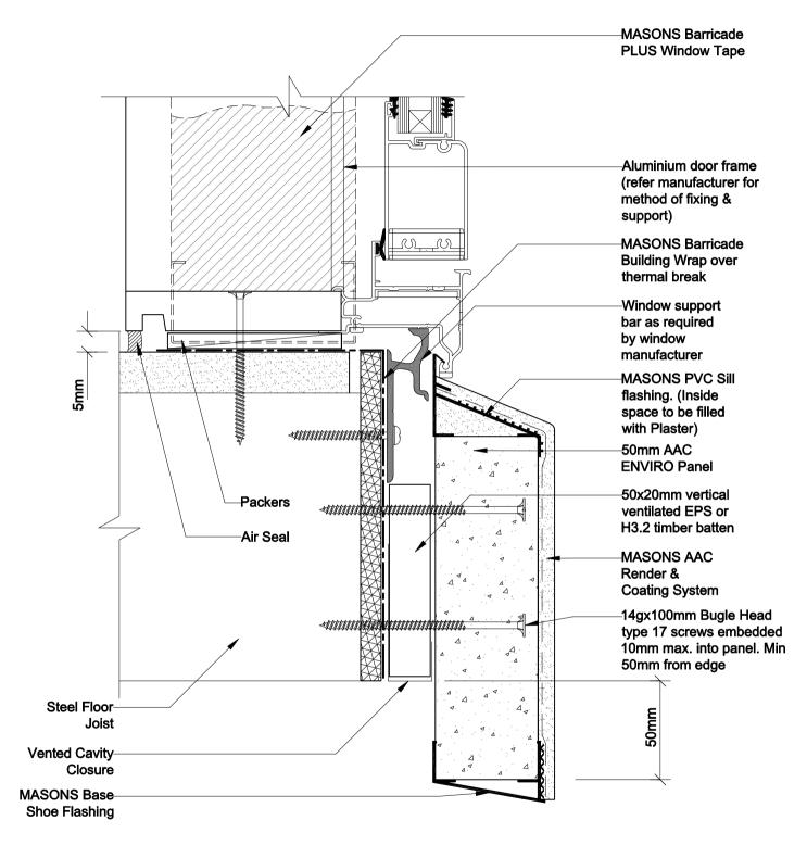
OPENING FLASHING -STEEL FLOOR DOOR SIII
