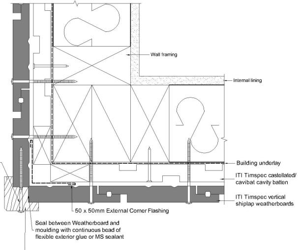
Nail P40 Moulding into side of both Weatherboards (only one nail shown for clarity) Stagger nails to avoid collision Drill pilot holes before nail to reduce risk of splitting.
