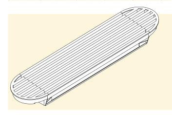
The SD single deflection blades can be retrofitted to existing installed LF grilles. The grille is removed from the mounting frame as described on the previous page and the SD simply clips on the rear surround.
