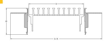
The same basic design as Model LD-1200 Linear Diffusers except that the Standard fixed, bar-type louvers are heavier 5.1 mm x 16mm as compared to 3.2 mm x 16mm.
