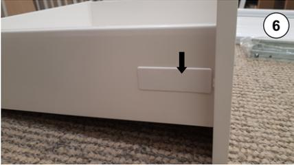
6 - Install the cover plate to hide fixings
