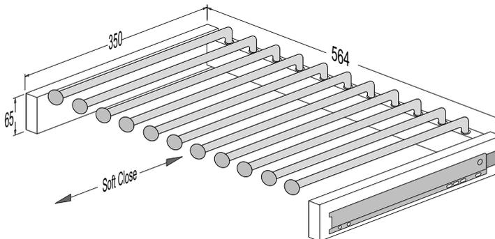
Note: If these Racks to be installed into Shelving units, the shelf must be ordered at 564mm wide
