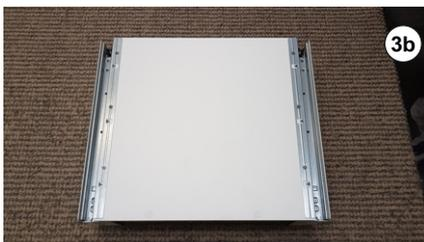
3a and 3b - Screw completed drawer sides to draw base.
