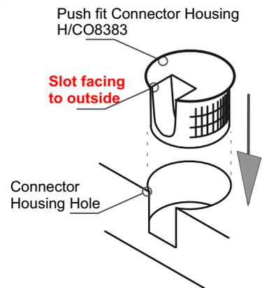
**Lockable Connector Housing** must be used on bottom shelves or in critical strengthening areas. Tap fit in place. After attaching shelf to the Connector Bolts the locking screws must be tightened (from below)
