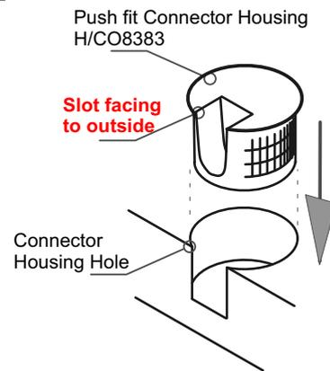
**Lockable Connector Housing** must be used on bottom shelves or in critical strenghtening areas. Tap fit in place. After attaching shelf to the Connector Bolts the locking screws must be tightened (from below)
