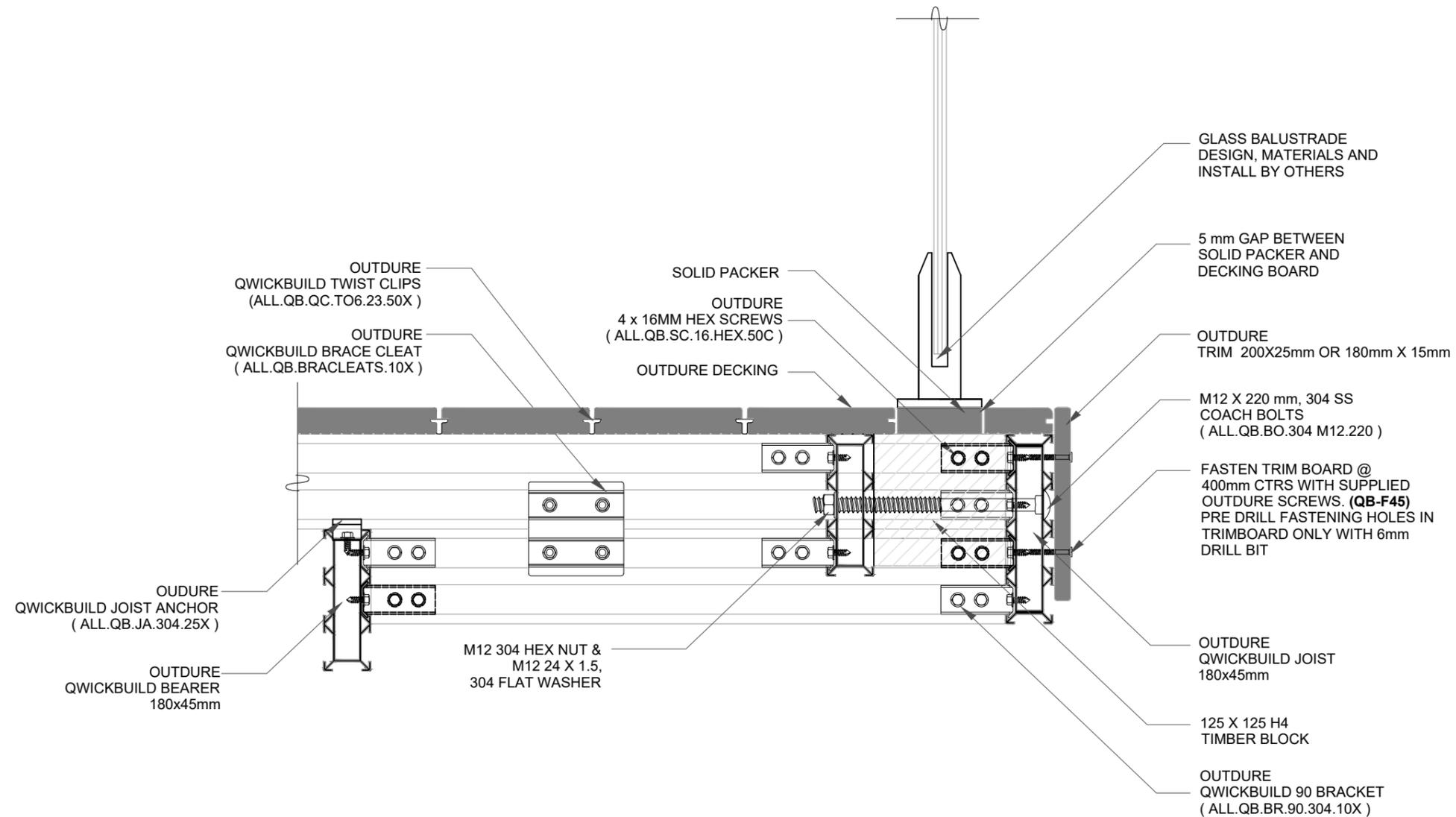
**1 QB-G3. BALUSTRADE PERPENDICULAR TO JOIST DIRECTION FOR 90mm JOIST ( SECTION VIEW 1 )**
