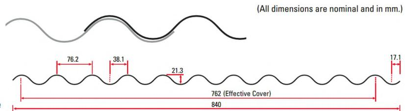
Acceptable Solution E2/AS1 provides for corrugate profile roofing with a minimum crest height of 16.5 mm.
