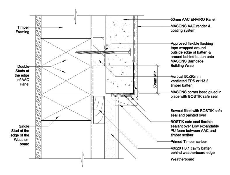
**AAC ENVIRO PANEL / WEATHER BOARD VERTICAL JUNCTION** Detail 39 Scale 1:2 **Plan View**
