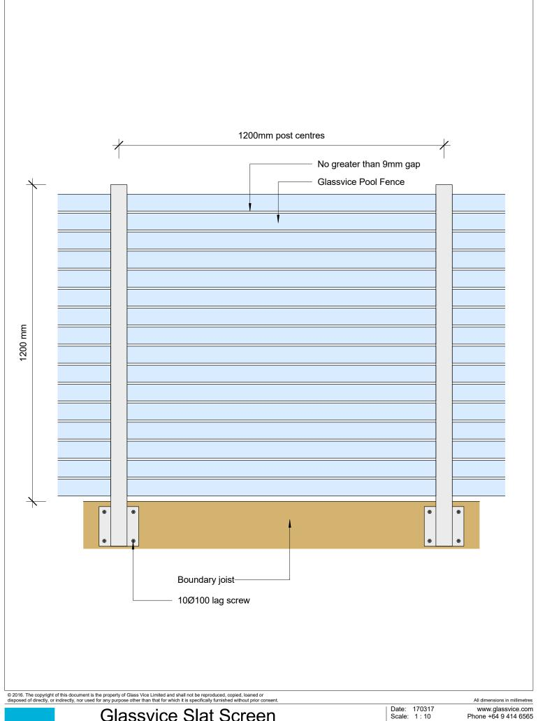
Glassvice Slat Screen Pool Fence TImber Side Fix Elevation
