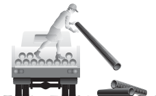
Incorrect way to off-load
