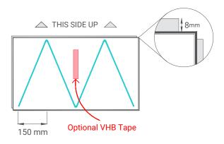
For all DumaWall XL panels, the adhesive should be applied as a continuous 5 mm bead in a zig-zag pattern at 300 mm centres. 300 mm
