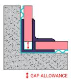
Note: Gap allowance may be needed for installing the last tile/panel in a row or considering that DumaWall XL has the ability to expand/contract up to 1 mm/m length.
