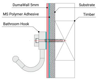
Where the tile/panel is required to be waterproof, BRANZ recommends the following approach: Identify, mark, and predrill the fixing location. Before inserting the fixing, fill with sealant. Apply sealant to the back face of the plate or bracket before fixing through the DumaWall to the framing.
