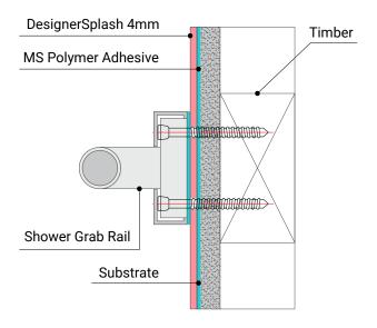
Where the panel is required to be waterproof, BRANZ recommends the following approach: Identify, mark, and predrill the fixing location.
